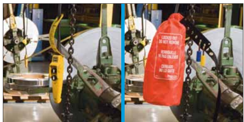
Hoist Control Lockout
