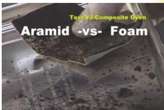
In contrast, PVC foam liners (and/or thermal enhancements) are embrittled and structurally unsound.
