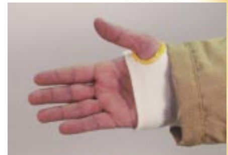
Overcast thumbhole is bulky and even the most careful craftsmanship will not be able to catch all the compromised knit stitches.
