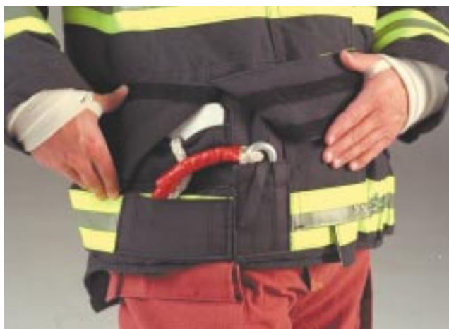
With both flaps raised, the retaining slots for the hook and stop plate are evident.
