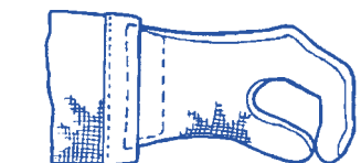
Standard Cuff Design Allows Glove Liquid Entry In Some Hand Positions
