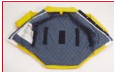
Coat prepared to receive the Lumbar Belt. The center strips are pile velcro (not hook, which would irritate your back and potentially pull your shirt when coat was worn without the lumbar in place). The two strips on either side of the pile, hook and loop are elastic pieces covered with Nomex knit.
