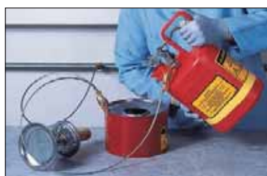
Grounding with antistatic wires
